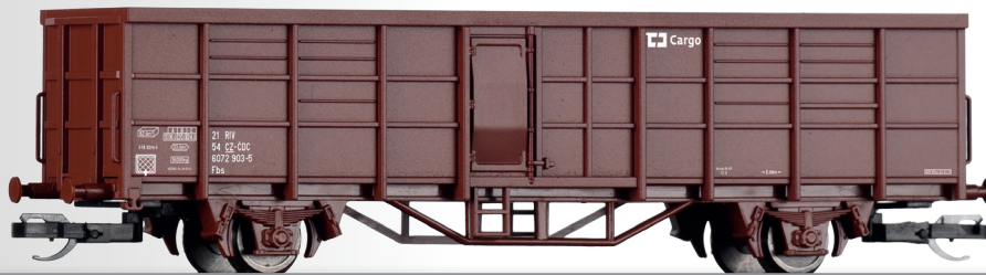
START-Offener Güterwagen Fbs der ČD Cargo START-Open car Fbs of the ČD Cargo
